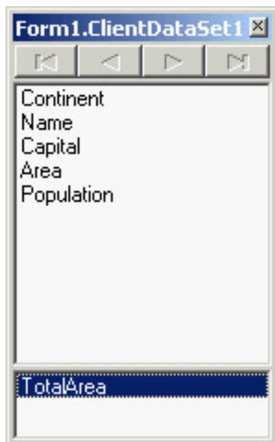
Figure 13.17: The bottom portion of a ClientDataSet's Fields Editor displays aggregate fields.
