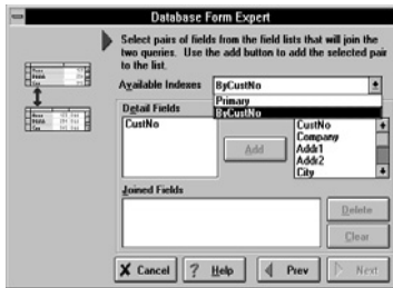
Figure 2.4 Linking fields in a master-detail form
