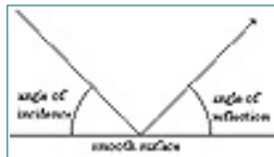
Figure 5-5. Specular Reflection Angles.
