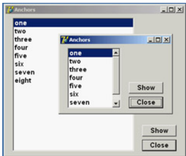
Figure 5.8: The controls of the Anchors example move and stretch automatically as the user changes the size of the form. No code is needed to move the controls, only proper use of the Anchors property.
